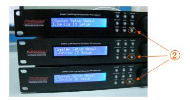
2: Each processor has to be set up a different ID number. (You can see the manual how to set up the ID number).
